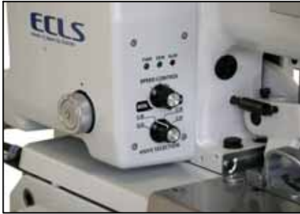
Control panel for error check, selection knob for C/B, C/A and sewing speed 1,000 ~ 2,000spm.
