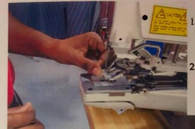
Put the button in the clamp—the holes are squared off with the machine.
